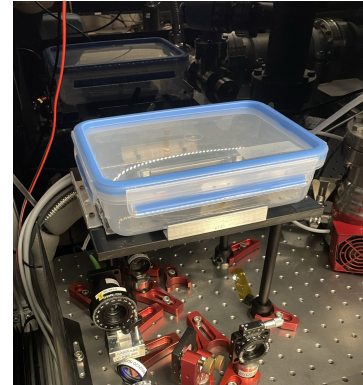
Figure 5.7: Nanofiber in transportation box on the fiber testing table after the lid was swapped and the fiber prepared.
