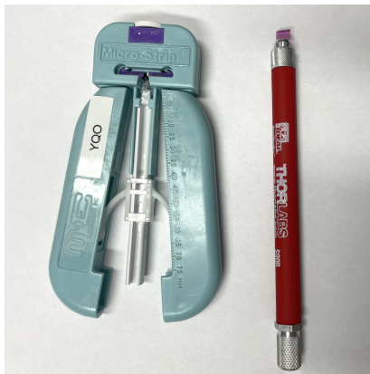
Figure 5.3: Mechanical fiber coating stripper and a fiber scoring pen
