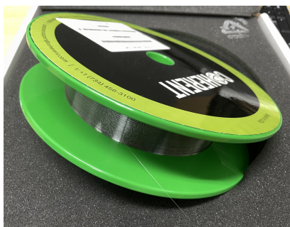
Figure 5.1: Bare Coherent 405-HP fiber on a fiber spool
