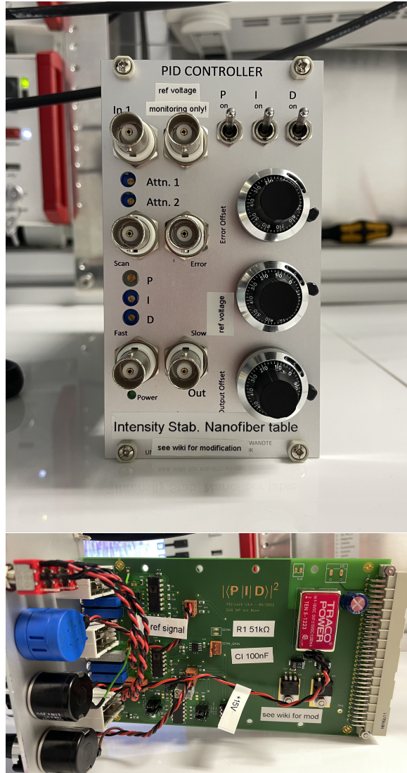
Figure 4.9: Proportional–integral–derivative (PID) controller built by the electronics workshop of the group and modified by me. The PCB in the bottom shows the modifications. The inputs and potentiometer on the front panel are relabeled for their modified use.
