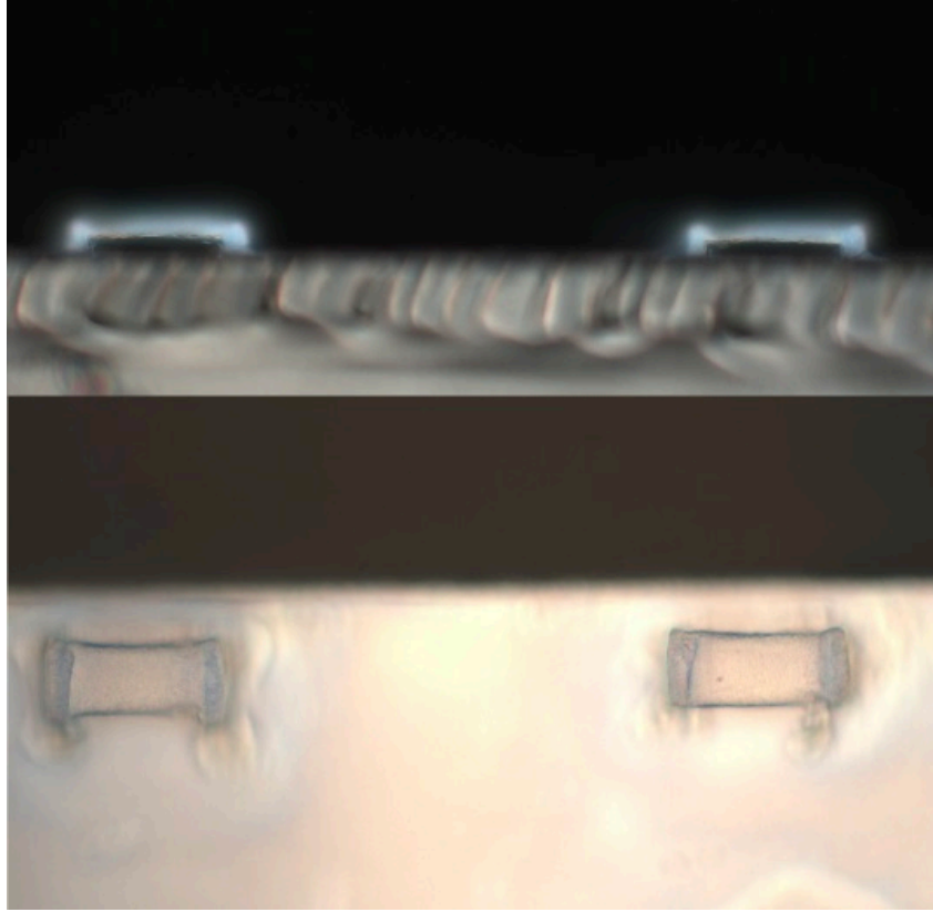
Figure 4.19: In this image, the results are shown for membranes with an increased height from 10\text{ }\mu\text{m} to 19\text{ }\mu\text{m} and a thickness of 2.5\text{ }\mu\text{m} , which were plasma ashed at 100% power for two hours. The top image, taken from a 90^\circ angle with the focus on the IP-S layer, shows that the layer is reduced in thickness while the membranes remain planar. The bottom image, taken from a top-down perspective, reveals the roughly homogeneous surface of the GP-Silica membrane and that the contrast of the IP-S membrane is significantly reduced.
