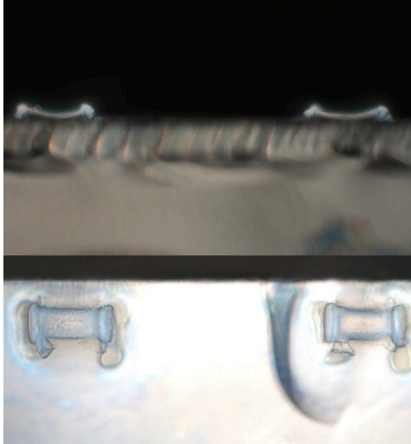
Figure 4.21: In this image, combined membranes that were plasma-ashed prior to shooting are shown, once from a 90^\circ angle ( top ) and once from a top-down perspective ( bottom ). From the 90^\circ perspective, the remnants of the IP-S membranes appear as thin, transparent, frayed layers, visible in focus on the left membrane. Additionally, the membranes have been pressed down at the center to the substrate, whereas they were planar before. From the top-down perspective, it can be observed that the optical properties have not changed significantly after shooting, and there are no indications of membrane contraction. Based on these observations, it can be concluded that the membranes were not fully, or possibly not at all, sintered.
