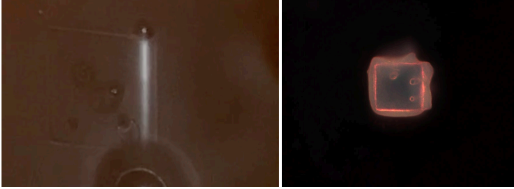
Figure 3.9: Left: Inside the Nanoscribe, the laser beam induces bubbles in the resin due to overheating. Right: Developed overexposed cube printed for the first time on a dielectric Bragg mirror. The bubbles remain visible even after development, and additional leakages have appeared.
