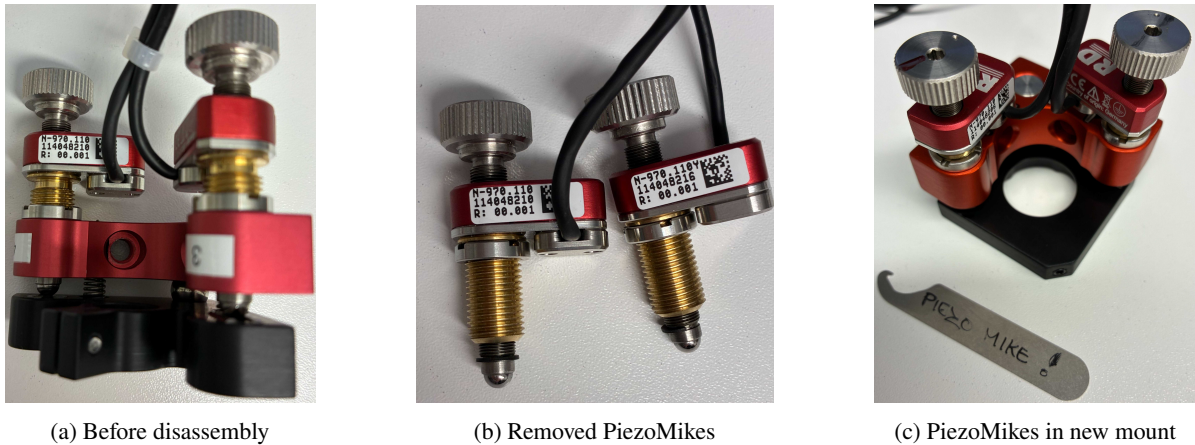
Figure 2.6: Before and after images of the mirror mount replacement for the PiezoMikes
